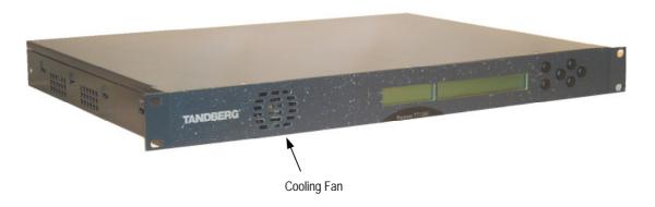
Figure 6.1: Cooling Fan Location
